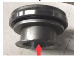
Then apply high pressure wheel bearing grease to the contact surface of the clutch fork and throw-out bearing interface surface before installing – Red arrow shown below.
