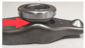
BE SURE THE INSTALLATION OF THE THROW-OUT BEARING ONTO THE CLUTCH FORK IS CORRECT.
