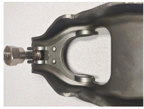
Above is the pivot stud correctly attached to the fork (not attached to the bell ) \*grease not shown here
