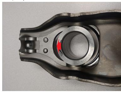
Shown above is the **CORRECT** way to install the bearing. The spring-ends must be under the bearing surface with the red arrow. The red arrow simulates the detent bump position when installed.
